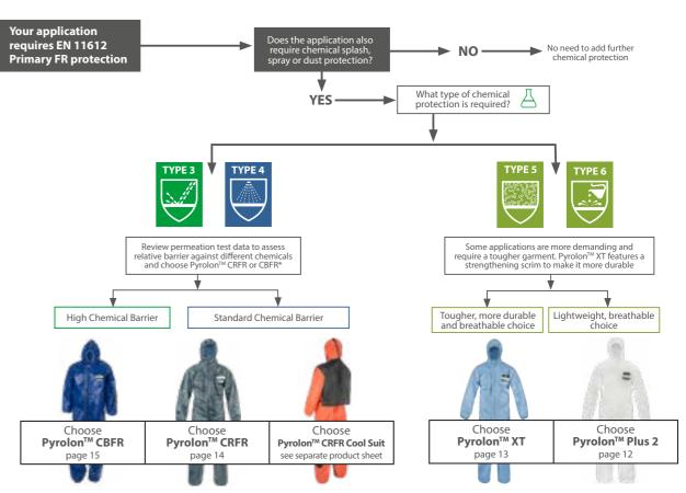
• Note: that permeation test data is not an indication of safe-wear time and should not be used as such.
