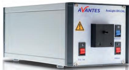
For calibrations in the ultraviolet and visible range (200-1099 nm), the AvaLight-DH-CAL is the best solution. This source can be used with all AvaSpec spectrometers to calibrate for absolute spectral intensity. It is supplied with a built-in diffuser, a cosine corrector (CC-VIS/NIR) with SMA adapter and the calibration files in ASCII format.
