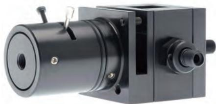
Have the most flexible setup with the combined cuvette holder, attenuator and filter holder. You can control the light throughput from 0-100%, which can be fixed with a set screw. Use the cuvette holder for any cuvette up to 10x10 mm and add half inch diameter (12-13 mm) filters of 1-8 mm thick.
