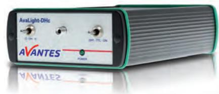
Get the best out of two worlds with the AvaLight-DHc. It has both a deuterium light source and a halogen light source, providing you with adequate light between 200 and 2500 nm for nearly all absorbance chemistry applications. Deuterium emits light between 200 and 550 nm, where the halogen takes over up to 2500 nm. Coupling this lightsource to the rest of your spectroscopy system is easy with the SMA connector.
