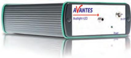
The AvaLight-LED is a compact, low-cost light source meant for fluorescence applications. It produces continuous or pulsed spectral output at different wavelengths. Some standard excitation wavelengths are shown in the table on this page, but other wavelengths are available upon request. The sources have an SMA-905 connector to couple to fiber-optics. Please note that the power supply (PS-12V/1.0A) has to be ordered separately.
