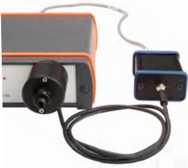
For accurate results during a transmission, absorption, reflection, irradiance or color measurement at different integration times, a good dark measurement is necessary. Taking this dark measurement often leads to having to undertake manual actions, like covering the sensor or switching off the light. This might prove to be problematic with certain applications because of the time and place or operator restraints.
