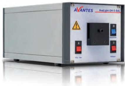
The AvaLight-DH-S is a powerful deuterium halogen source, but like any unbalanced deuterium halogen source it does have a very dominant alpha peak at 656 nm. This is why Avantes developed the DH-S-BAL, in which this peak is drastically reduced by a dichroic filter. This means less power, but an increase in the dynamic range of a factor 20. A comparison spectrum, which is taken with a standard AvaSpec-ULS2048CL, is shown on the next page.
