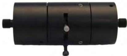
For all UV-VIS-NIR applications and ATT-INL-EXT setups where light intensity has to be reduced, Avantes offers the inline fiber-optic attenuator (ATT-INL-EXT) and the direct attached fiber-optic attenuator (ATTDA). This device is an iris attenuator which controls light throughput to avoid detector saturation. The ATT-INL-EXT is coupled between two SMA terminated fiber-optic cables, whereas the ATT-DA can
