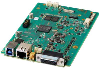
The AS-7010 is the all new electronic platform and the base for Avantes' future spectrometer models.
