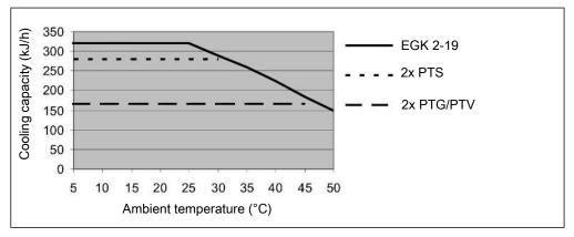
Note: The limit curves for the heat exchangers exchanger apply to a dew point of 40  $^{\circ}$ C.
