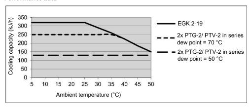
Remark: The limit curves for the heat exchanger apply to a dew point of 70 °C under standard conditions per DIN EN 15267-3:2008-03 and to a dew point of 50 °C under operating conditions.
