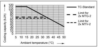
Note: The limit curves for the heat exchangers MTV-2 and MTG-2 apply to a dew point of 50 °C.
