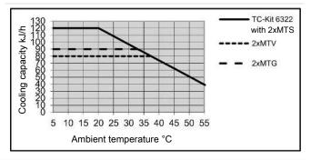
Note: The limit curves for the heat exchangers exchanger PTG, MTG, PTV or MTV apply to a dew point of 50 °C.
