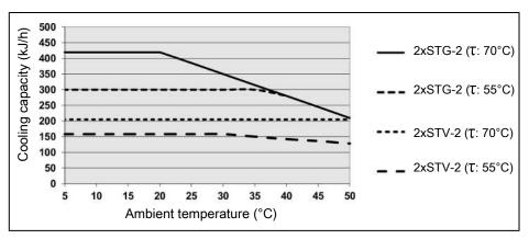
Note: The limit curves of the heat exchangers apply to different dew points ( $\tau$ ), see legend.
