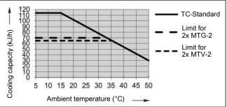
Note: The limit curves for the heat exchangers MTV-2 and MTG-2 apply to a dew point of 50  $^{\circ}$ C.
