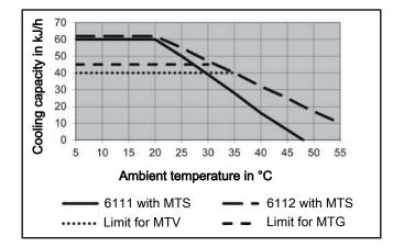
A selected outlet dew point of 10 or 15  $^\circ C$  shifts the curves 5 or 10  $^\circ C$  to the right.
