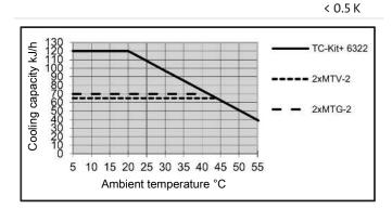
Note: The limit curves for the heat exchangers MTV-2 and MTG-2 apply to a dew point of 50 °C.
