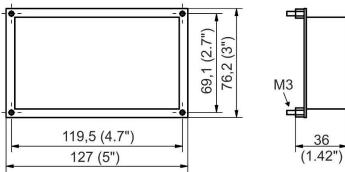
Power board (option expansion module 24 V)
