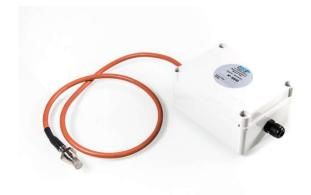
For the measurement in very hot environments or gas at high temperature, a special Zirconium dioxide (ZrO2) sensor  $_{is}$  used. In this case the 4-20mA transmitter is contained in a plastic container, while the sensor is positioned at the end of a 1 m long cable, and the probe containing the sensitive element is available in 3 different lengths: 28, 45, 55 mm.
