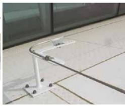
Kee Safety's **POSTANKA** range of fabricated, hot dipped galvanised anchors are designed using a standard calculation program to the requirements of EN 795 Class A2 or OSHA's 5000 lbs (22.2kN) requirement.
