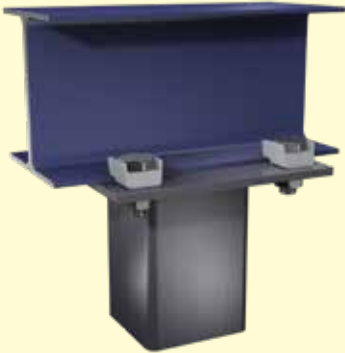
Column end plate to I-Section
