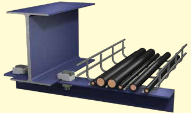
Cantilevered angle support for running cable tray
