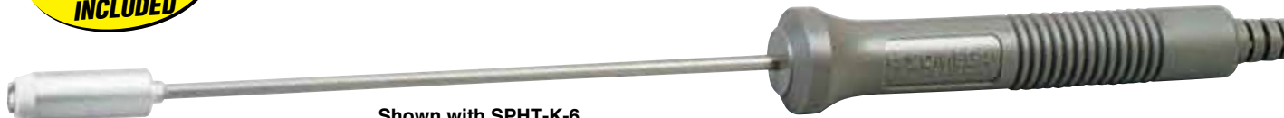
Shown with SPHT-K-6, 6" long K Type surface probe included.
