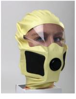
A personal respiratory protective device intended for self-rescue during emergency situations involving chemical spills. The KIMI mask provides users with short-term respiratory protection against organic gases and vapors with a boiling point higher than 65°C, certain inorganic gases and vapors, Sulfur Dioxide and other acidic gases and vapors, Ammonia and Ammonia derivatives.
