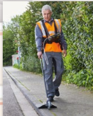
Walking on a curb following exactly the crack between stone and asphalt, thanks to the Mono-wheeler Carpet Probe.
