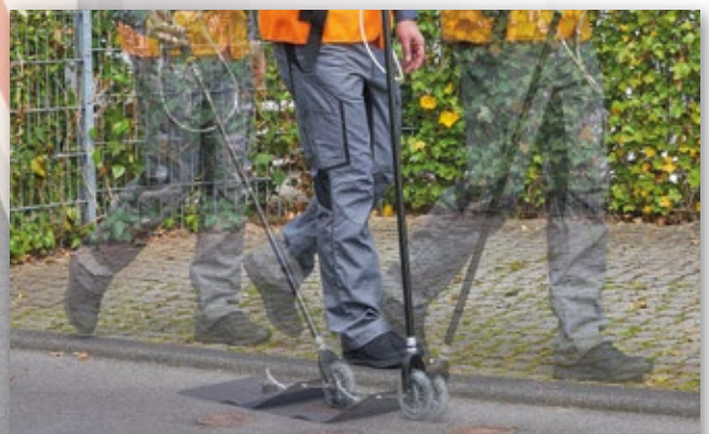
Stopping the Carpet Probe an extra second on top of manhole covers without interrupting your walking pace.
