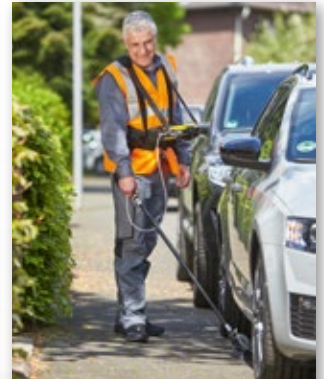
With a twist of the wrist you can turn the Carpet Probe backwards and easily search under cars or other obstacles.
