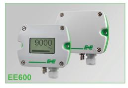
EE600 stands for full flexibility. Using DIP-switches on the electronics board, the user can select the pressure range, the output signal, the time constant as well as the units and the backlight of the large, graphic display. The user can easily perform a zero and span point adjustment with push buttons on the electronics board.
