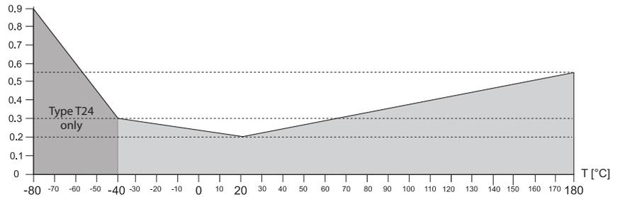
Temperature dependence of electronics, typ. ±0.001°C/°C
