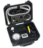
The Interceptor® Plus Pressure Test Kit includes everything you need to conduct regular tests including connection hoses and valves, air blower and magnahelic pressure gauge.
