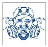
2. Pull the ends of the six straps to adjust tightness, starting with the neck straps first, followed by the temple straps. Do not overtighten the head straps as this may deform the nose cup and narrow the inhalation air passage.
