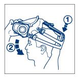
1. Fully loosen all six headstraps, then place the harness at back of head and position facepiece over the face.
